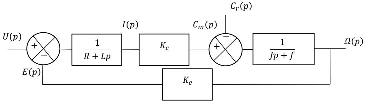
$$\Omega(p) = H_U(p)U(p) - H_{C_r}(p)C_r(p)$$
